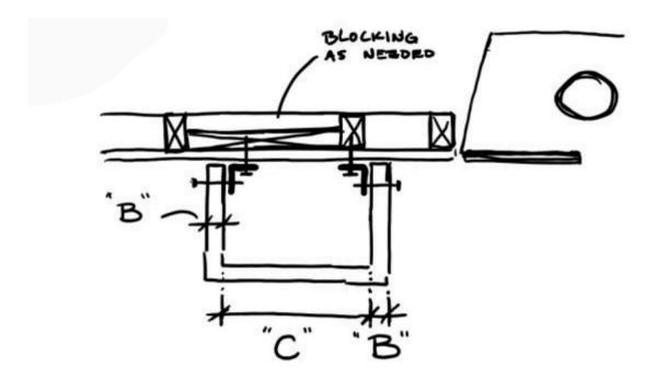
• **Step 6.** Install mounting brackets using 2 sharp point screws per bracket. When installing 2x2 mounting bracket to wall we recommend pre-drilling the bracket.
